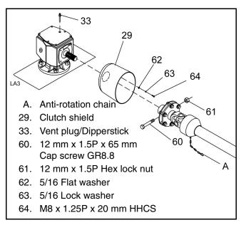
Figure 32. Slip Clutch Driveline Assembly
